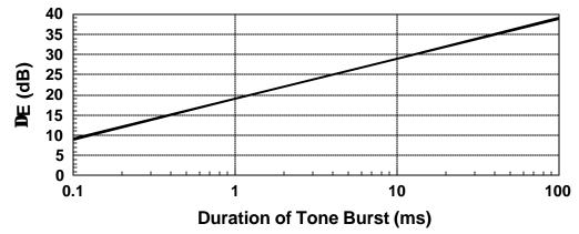
Figure 6. The amount of energy in dB that a tone burst would have over a dolphin echolocation signal of the same peak-to-peak amplitude.
