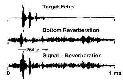
Figure 9. Target echo in reverberation at the dolphin's threshold of detection (from Au [8]).
