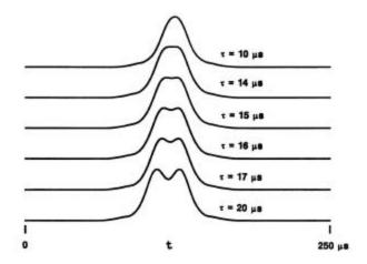
**Figure 13.** The normalized envelope of the cross correlation function of echoes from two point targets separated in time by  $\tau$  and the transmitted signal shown in the top left panel of Fig. 4 (from Au [5]).
