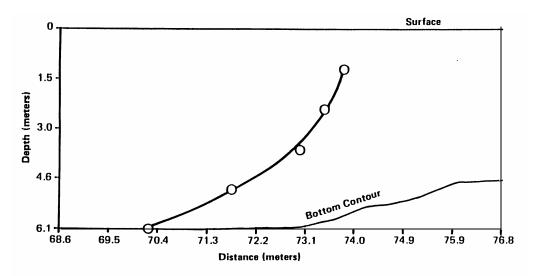
**Figure 8**. Target detection threshold as a function of target depth. The detection range when the 6.35cm diameter sphere laid on the bottom was approximately 70 m (from Murchison [7]).
