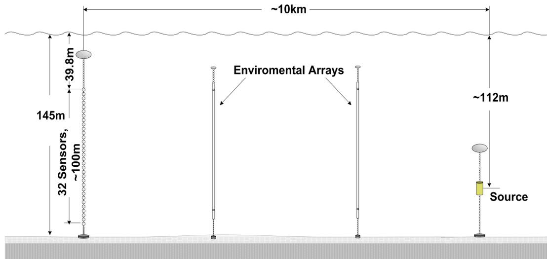
FIGURE 1. Experimental geometry for the South Florida Strait site.
