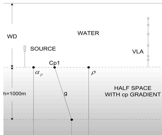
**FIGURE 5.** Geoacoustic model used for the South Florida Strait environment.
