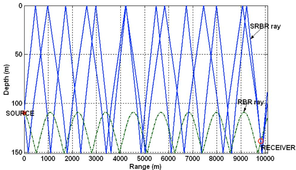
FIGURE 3. Illustration of RBR and SRBR rays from the source at 112 m.
