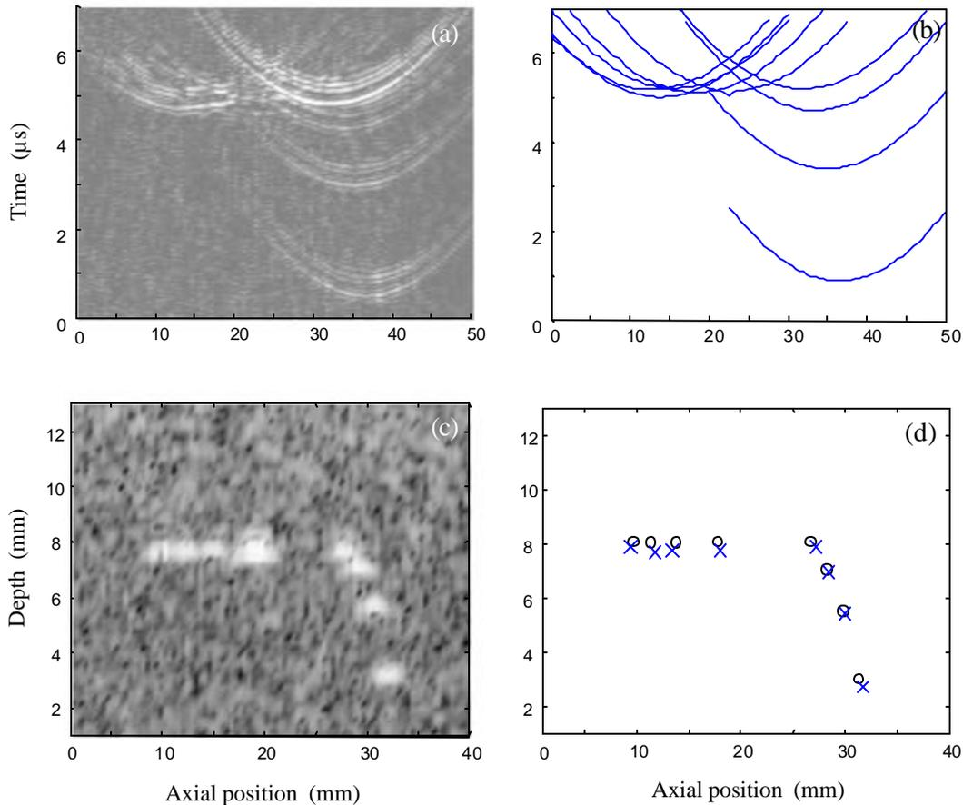
**FIGURE 3.** Target detection in a biological phantom. a) Signal received after a plane wave illumination, we can see some echoes of the targets with an important speckle noise from the phantom. b) Detection of the echoes of 9 targets. c) B scan image of the phantom. Due to the speckle noise, the smallest targets are difficult to resolve. d) Calculation of the targets positions from the detected echoes. The x are the measured positions and the circles are given by the furnisher of the phantom.
