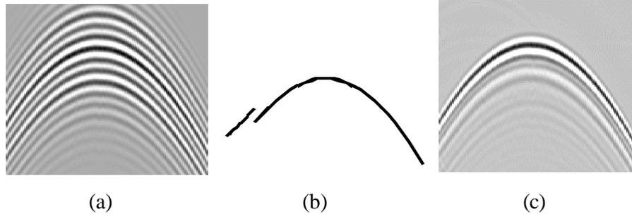
**FIGURE 2.** a) After the iteration of the time reversal the signal is enlarged. b) Selection of a wavefront only, this wavefront has a defect in the detection. c) After emitting this wavefront, we obtain a narrow pulse, in this narrow pulse there are not defects in the identification of the wavefront.
