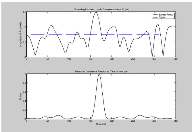
**Figure 2. A sample temporal weighting function reflecting a single path in an acoustic channel. The coherence time (75% confidence level) for this path is specified to be 20 ms.**
