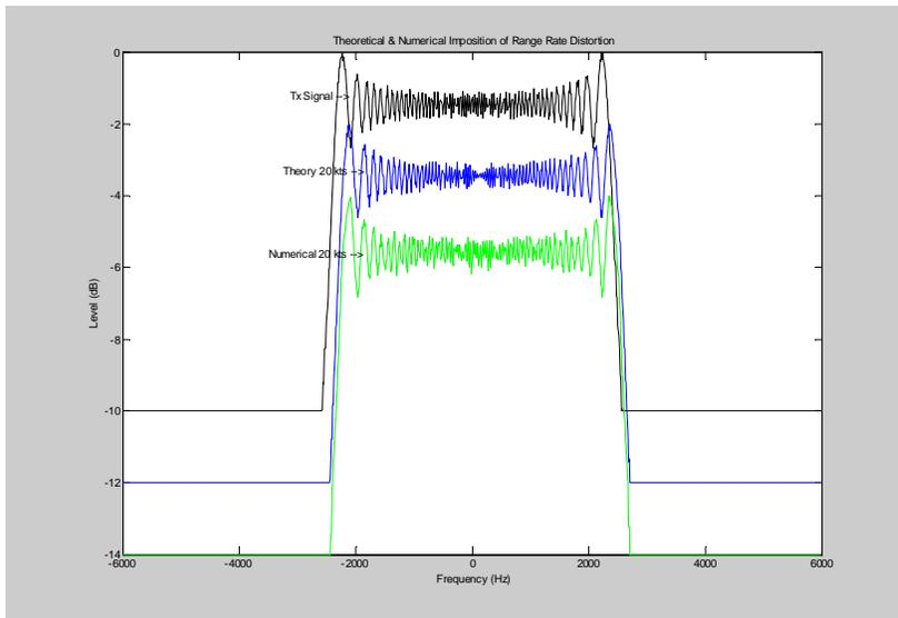
**Figure 5. Comparison of the Power spectra of the original transmitted LFM (upper trace), and the “received” signal perturbed by 20 kts of range rate. The middle trace reflects a theoretical model, while the third trace reflects a numerical imposition. They are virtually identical. The vertical offsets in the plots are included only to clarify the presentation.**
