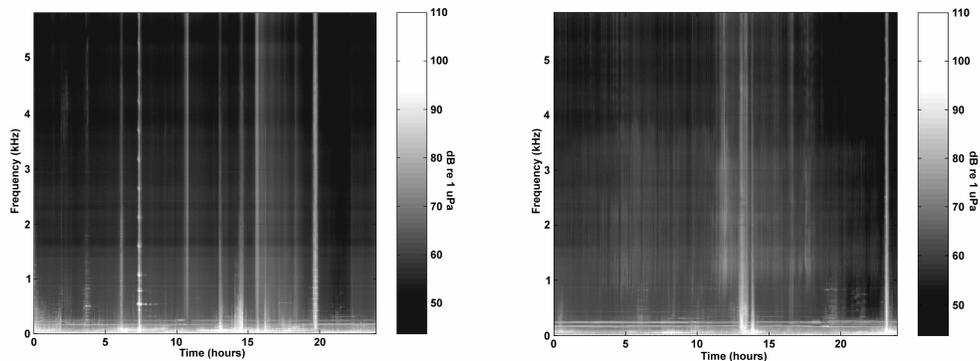
**FIGURE 4.** Spectrograms of the ambient noise before (left) and during (right) Tropical Storm Barry.
