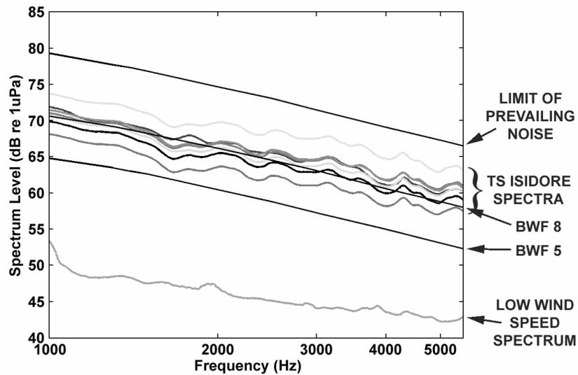
**FIGURE 3** Illustration of the ambient noise results for EARS3 during Tropical Storm Isidore superimposed upon the results from Wenz [1] for Beaufort Wind Force 5 and 8. Also shown are the upper limit of the prevailing noise from Wenz [1] and a low wind speed spectrum for comparison.
