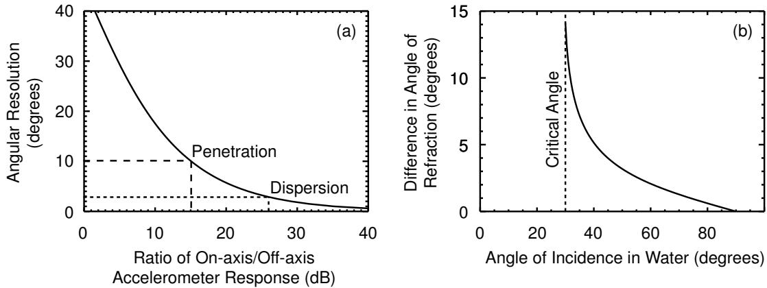
**FIGURE 1.** (a) Estimated angular resolution as a function of the ratio of on-axis to off-axis accelerometer sensitivity. Penetration (long dash) and dispersion (short dash) measurement requirements are superimposed. (b) Difference in angle of refraction for sediment/water sound speeds ratios of 1.15 and 1.09 as a function of grazing angle.
