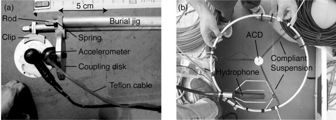
**FIGURE 2.** (a) Pair of uni-axial accelerometers mounted to coupling disks that are orthogonal to each other. The sensors are attached to the burial jig using clips on the edges of the disks. Springs temporarily fix the clips to the inner, square, rod of the burial jig. The sensors are released when the square rod is retracted. (b) The accelerometers are calibrated individually in water by mounting them on a frame using very soft springs. A hydrophone is also attached to the circular frame.
