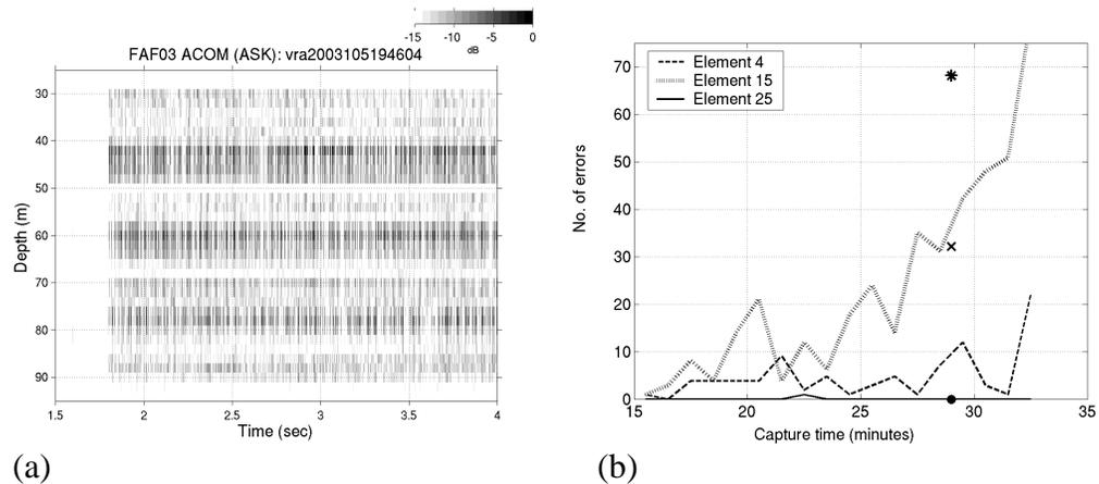
**FIGURE 6.** (a) The first 2 sec of measured binary ASK data to the three depths of VRA (42 m, 60 m and 78 m). (b) BER out of 4,900 bits as a function of time at three different focal depths using an incoherent binary ASK modulation. The results are from simulated ASK sequences based on 40-minute round-robin channel response data and decoded using passive time reversal. The dots denote the BER of active time reversal ASK communication data.
