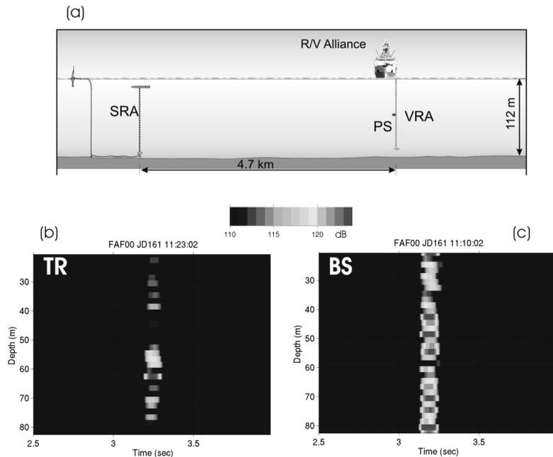
**FIGURE 1.** (a) Experimental configuration for reverberation measurements carried out north of Elba Island off the west coast of Italy. The PS was deployed from the R/V Alliance at 60 m depth and 4.7 km range away from the SRA. The PS pulse was a 100-ms long pulse at 3.75 kHz. (b) TR focusing recorded by the VRA near the PS. For comparison purposes, (c) shows a BS transmission received by the VRA which fills the water column.
