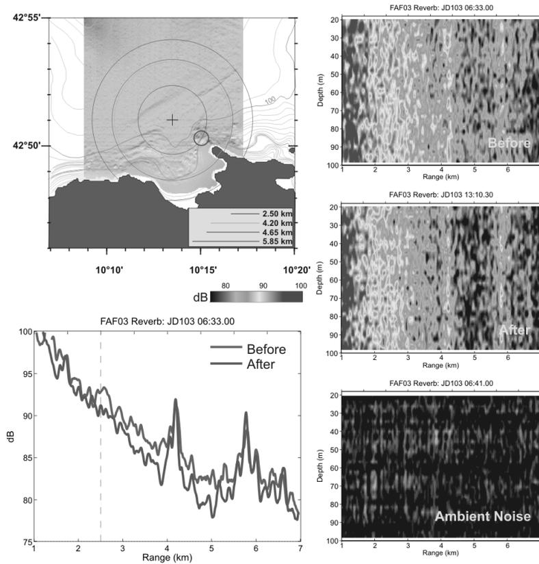
**FIGURE 3.** Experimental demonstration of reverberation nulling at 3.5 kHz. Note the reduction of reverberation level at the intended 2.5 km range as compared to the original reverberation from a broadside transmission (BT) of the SRA (bottom left). Right column: Reverberation level in time and depth along with ambient noise level.
