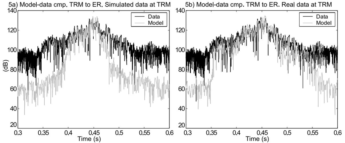
**FIGURE 5.** Model-data comparison of the field transmitted from the TRM and received by the echo repeater (ER). In the modeling result (Fig. 5a) the field transmitted is either simulated (Fig. 2a) or measured (Fig. 2b). The result using the measured signal includes noise recorded during the forward propagation phase, then time-reversed and retransmitted from the TRM. This noise contribution is not modeled.
