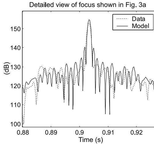
**FIGURE 4.** A more detailed view of Fig. 3a during a 50 ms time period spanning the focus. Model-data agreement is good to within a few dB at the focus.
