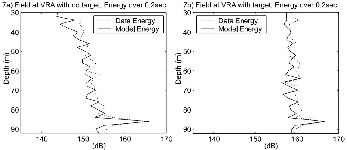
**FIGURE 7.** Comparison of energy received on the VRA over a 0.2 s time window centered at the signal's maximum peak. Left: model-data comparison with no target present. Right: model-data comparison with the target. Measured data energy is always higher than model prediction due to unmodeled noise, as in Figures 5 and 6.
