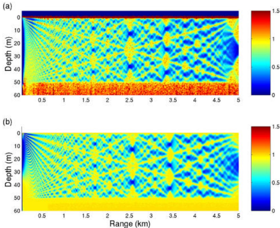
**FIGURE 4.** Comparison of (a) PE simulation for the scintillation index obtained by averaging over the results for 1000 rough surface realizations with (b) transport theory result.
