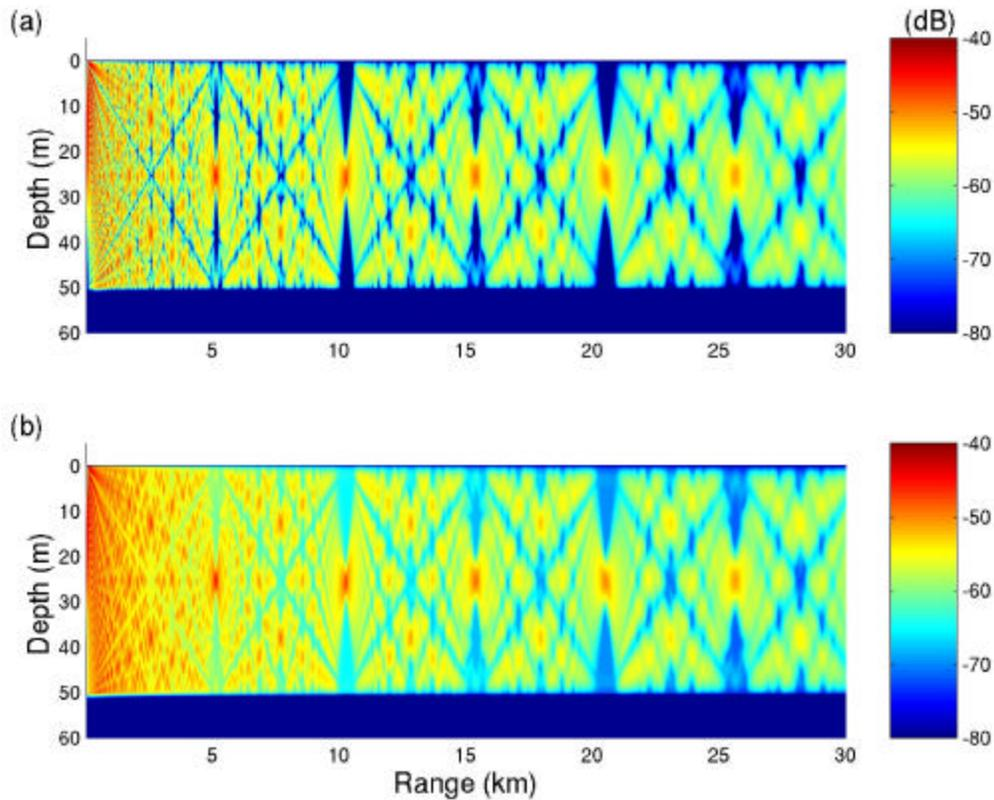
**FIGURE 2.** Transport theory results for coherent intensity (a) and total intensity (b) obtained in the Dozier-Tappert approximation.
