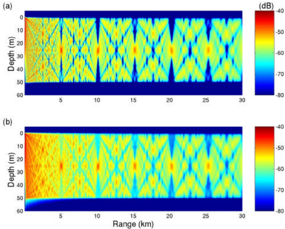
**FIGURE 1.** PE simulation for coherent intensity (a) and total intensity (b) obtained by averaging over the results for 50 rough surface realizations.
