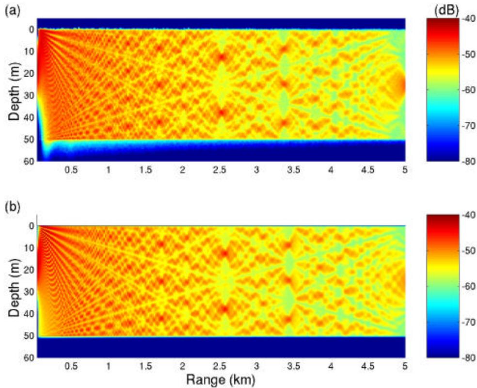
**FIGURE 3.** Comparison of (a) PE simulation for total intensity obtained by averaging over the results for 50 rough surface realizations with (b) transport theory result.
