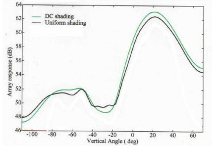
FIGURE 1. Measured vertical array response in deep water at 4.5 kHz.
