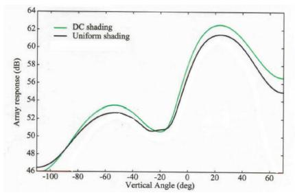
FIGURE 2. Predicted vertical array response in deep water at 4.5 kHz.
