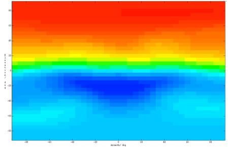
FIGURE 5. Measured ambient noise vs horizontal and vertical angle at 20kHz.
