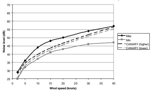
FIGURE 4. General bounds of measured omni directional noise and CANARY predictions 20 kHz.
