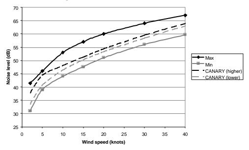
FIGURE 3. General bounds of measured omni directional noise and CANARY predictions 5 kHz.
