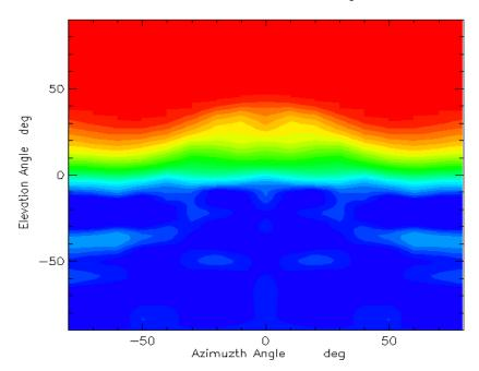
FIGURE 6. Predicted ambient noise vs horizontal and vertical angle at 20kHz.
