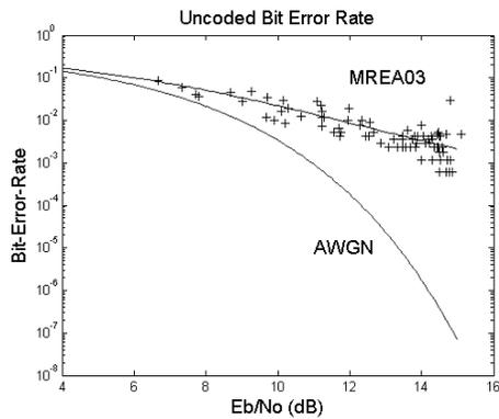
**FIGURE 5.** Uncoded Bit-Error-Rate: MREA03 Channel vs. AWGN Channel.
