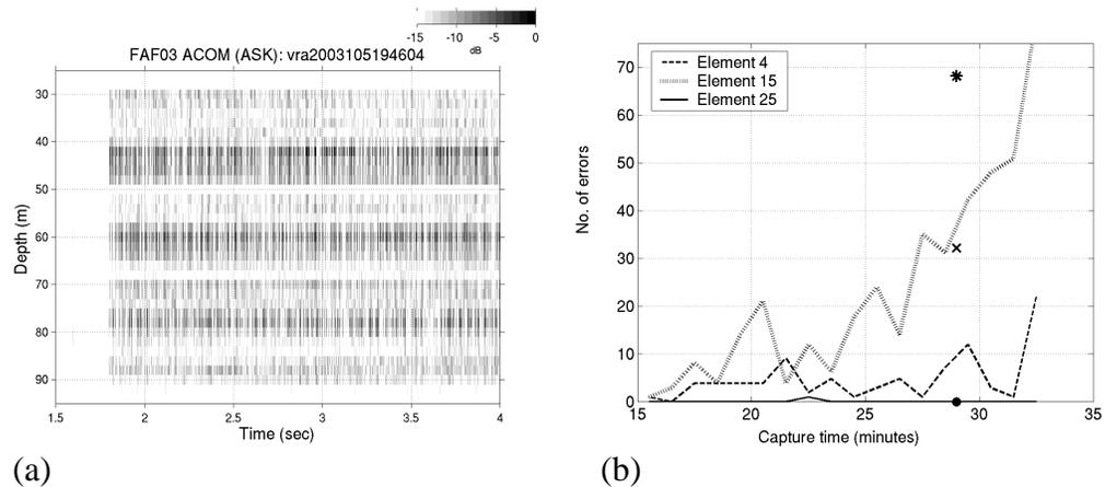
**FIGURE 6.** (a) The first 2 sec of measured binary ASK data to the three depths of VRA (42 m, 60 m and 78 m). (b) BER out of 4,900 bits as a function of time at three different focal depths using an incoherent binary ASK modulation. The results are from simulated ASK sequences based on 40-minute round-robin channel response data and decoded using passive time reversal. The dots denote the BER of active time reversal ASK communication data.
