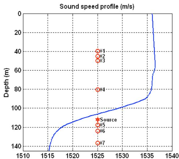
FIGURE 2. Sound speed profile, and locations of source and receivers in the water column.
