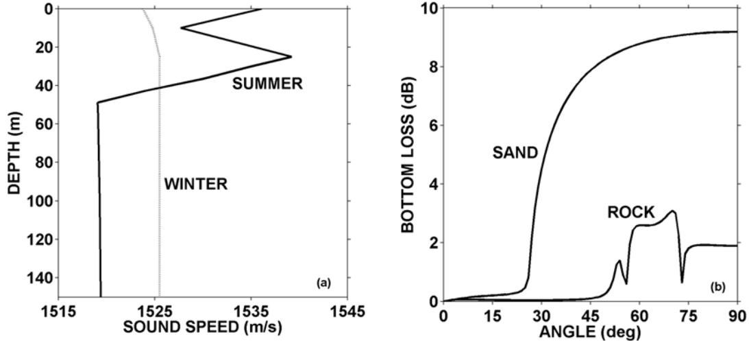
**FIGURE 1.** (a) Sound-speed profiles assumed in this study. (b) Bottom loss vs. angle at 3.5 kHz for rock and sand using REFLECT.
