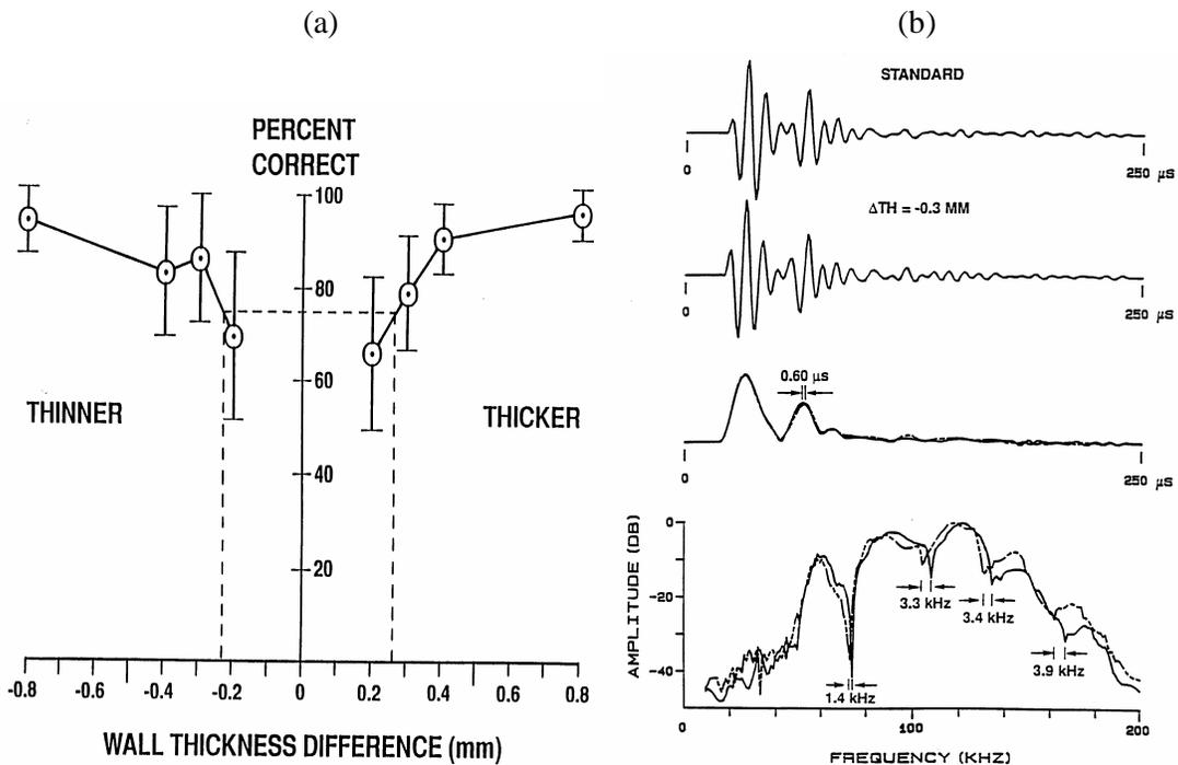
**Figure 12.** (a) Dolphin wall thickness discrimination performance, (b) Echo waveform, waveform envelope, and frequency spectrum for the standard and comparison target having a wall thickness difference of  $-0.3$  mm. The dashed envelope and spectrum curves are for the comparison target (from Au and Pawloski [11]).
