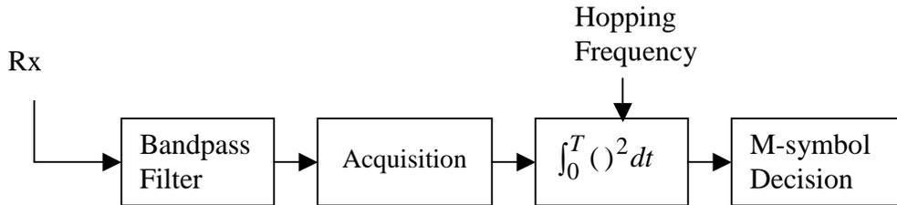
**FIGURE 4.** FH MFSK Energy Detector
