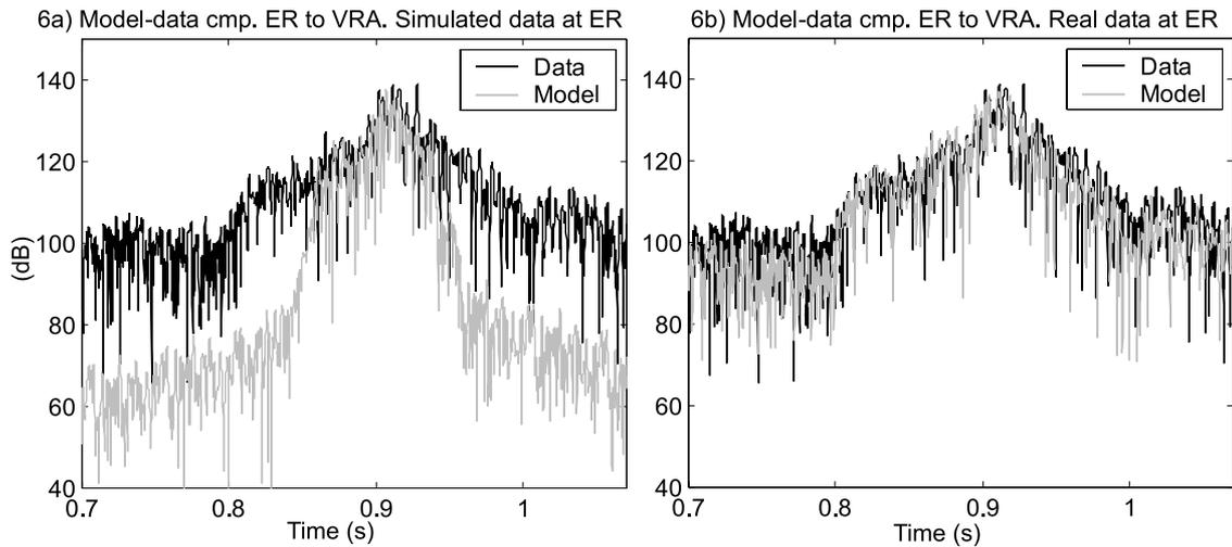
**FIGURE 6.** Model-data comparison of the field transmitted from ER to VRA, showing the received field that includes scattering from an insonified target. The ER gain simulated a target with an approximate TS of 60 dB. As in Fig.5, there is a noise contribution present when the measured signal is used that is not accounted for in the purely modeled prediction. However, in the 100 ms period spanning the focus, agreement is within a few dB. The data are from a VRA hydrophone at depth 64 m.
