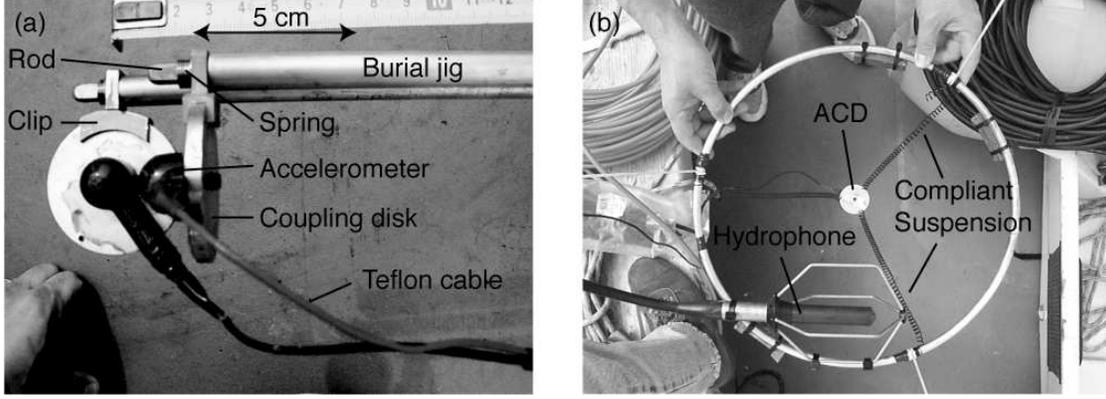
**FIGURE 2.** (a) Pair of uni-axial accelerometers mounted to coupling disks that are orthogonal to each other. The sensors are attached to the burial jig using clips on the edges of the disks. Springs temporarily fix the clips to the inner, square, rod of the burial jig. The sensors are released when the square rod is retracted. (b) The accelerometers are calibrated individually in water by mounting them on a frame using very soft springs. A hydrophone is also attached to the circular frame.
