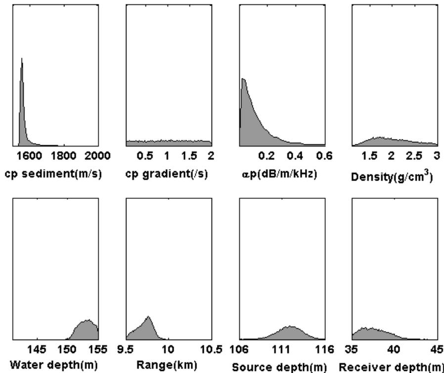
**FIGURE 6.** Marginal densities generated from the Gibbs sampling inversion for the geoacoustic and geometric model parameters.
