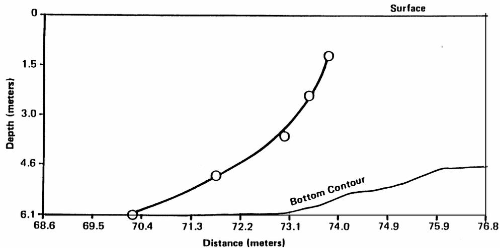
**Figure 8.** Target detection threshold as a function of target depth. The detection range when the 6.35-cm diameter sphere laid on the bottom was approximately 70 m (from Murchison [7]).
