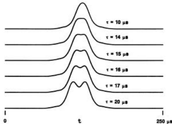
**Figure 13.** The normalized envelope of the cross correlation function of echoes from two point targets separated in time by  $\tau$  and the transmitted signal shown in the top left panel of Fig. 4 (from Au [5]).
