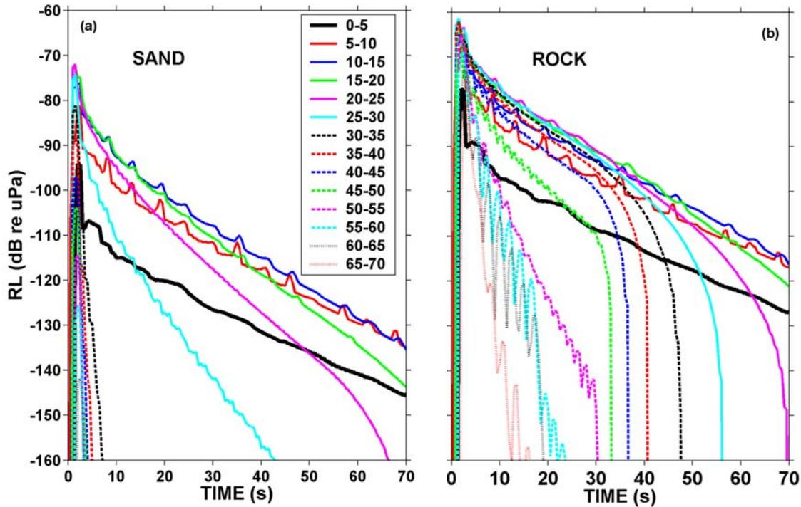
**FIGURE 4.** At 3.5 kHz for (a) sand and (b) rock: RL contributions by mean grazing angle in 5-deg bins for the  $\gamma_2 = 3.2$  and  $w_2 = 0.001 \text{ m}^4$  case. Summer profile and S-R at 75 m.
