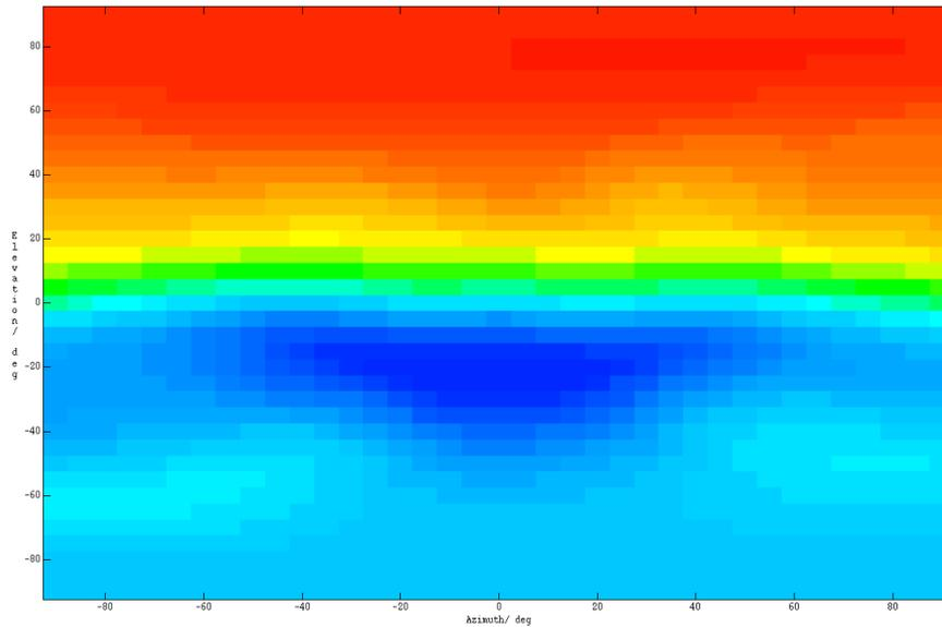
**FIGURE 5.** Measured ambient noise vs horizontal and vertical angle at 20kHz.
