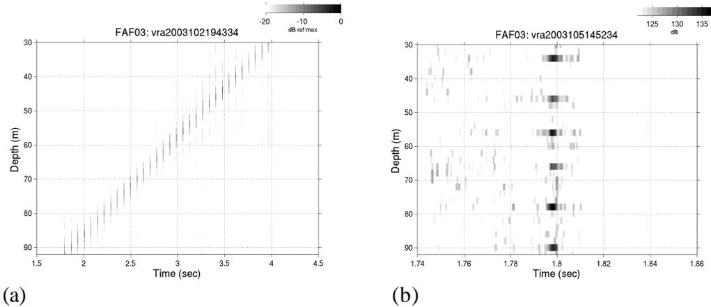
**FIGURE 5.** (a) Sequential focusing at every element of the VRA. (b) Simultaneous multiple focal spots at six depths.
