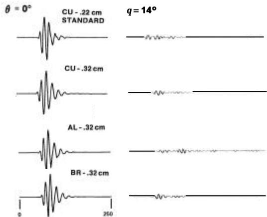
**Figure 11.** Examples of backscatter from the standard disk and some of the comparison disks used by Evans and Powell [9].
