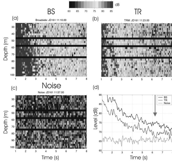
**FIGURE 2.** Measured backscattered field at the SRA: (a) BS transmission and (b) TR transmission. The ambient noise field is also displayed in (c) as a reference. (d) shows the corresponding reverberation level incoherently averaged across the upper SRA elements along with ambient noise level. The TR reverberation indicates about a 3 dB notch around 6.3 sec corresponding to the PS range of 4.7 km.
