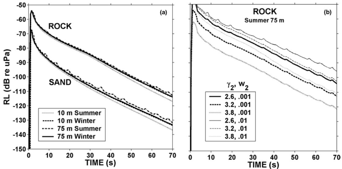
**FIGURE 3.** At 3.5 kHz: (a) RL for rock and sand for four scenarios for  $\gamma_2 = 3.2$  and  $w_2 = 0.001 \text{ m}^4$ ; and (b) RL for rock for six pairs of roughness values for one scenario.
