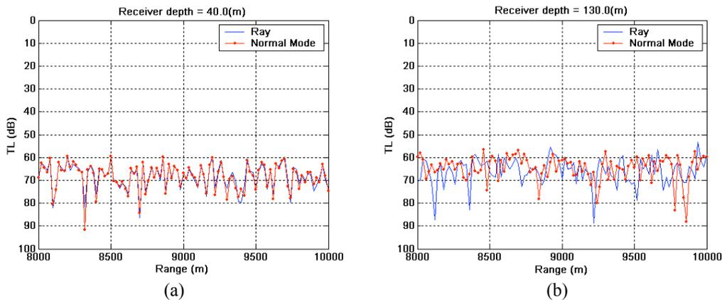
**FIGURE 4.** Comparison between TL calculated by normal mode and ray theory at different receiver depth (a) Receiver depth at 40 m; (b) Receiver depth at 130 m
