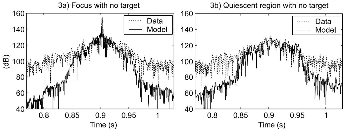
**FIGURE 3.** Comparison between data and model predictions for an unperturbed (no target present) focused field at two hydrophones on the VRA, one at the focal point at depth 86 m and the other in the quiescent region at depth 64 m.
