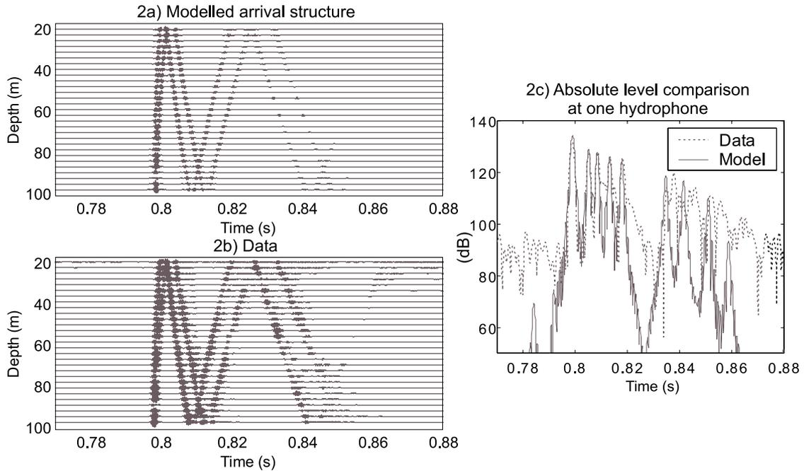
**FIGURE 2.** Modeled and measured impulse response of the waveguide given a point source at a depth of 86 m. The figure on the right shows the amplitude, in absolute level, of a representative arrival time series at one hydrophone (depth 67 m) on the VRA. The time envelope of pressure is shown. There is extremely good model-data fit for the first arrival and following four multipath echoes.
