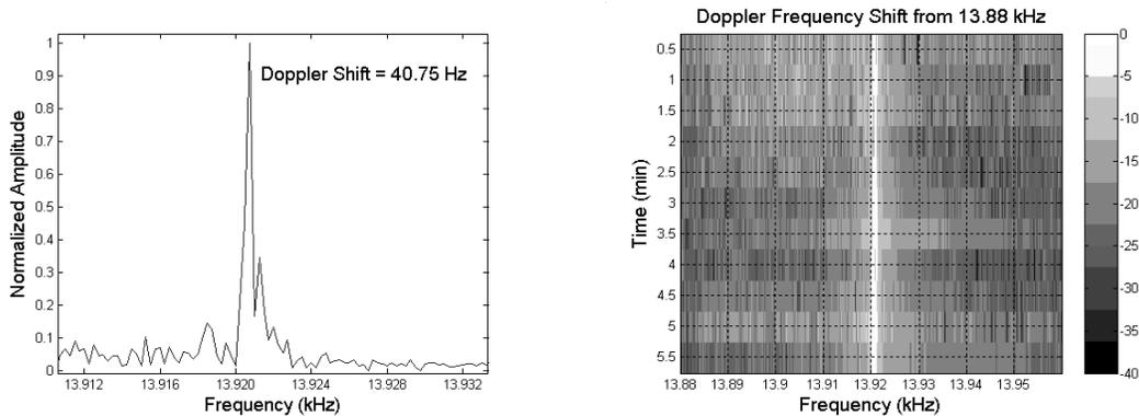
**FIGURE 2.** Doppler Frequency Shift Estimate. 2a: at a time instant (left figure) and 2b: vs. time (right figure).
