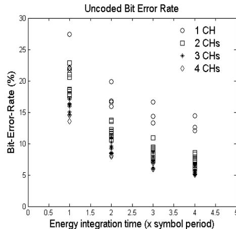
**FIGURE 8.** Multi-channel Combining Uncoded BER vs. Integration Time
