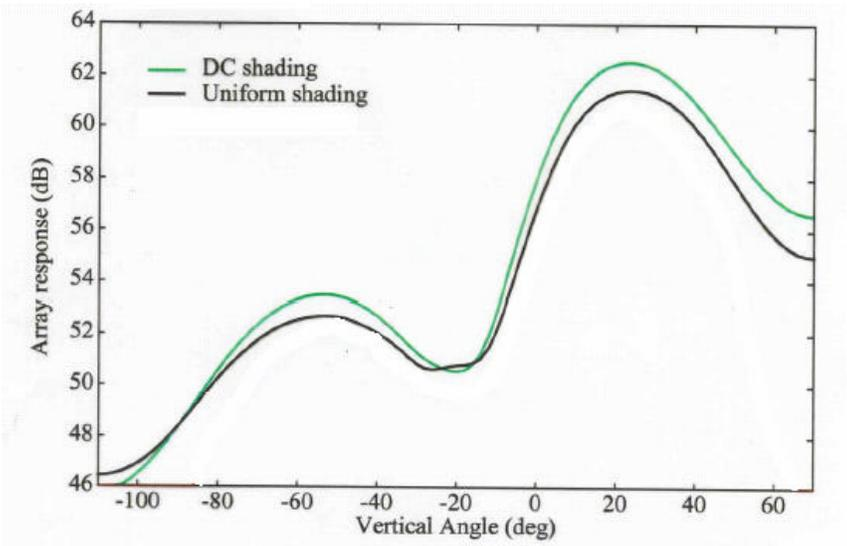
**FIGURE 2.** Predicted vertical array response in deep water at 4.5 kHz.
