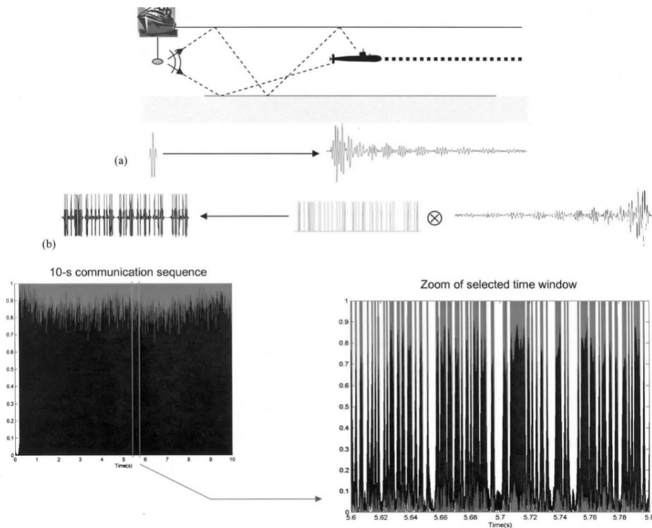
**FIGURE 7.** Synthetic, horizontal aperture communications. (a) Channel response due to a single bit. (b) Communication sequences convolved with a time-reversed version of the channel response. The bottom plots show decoded sequences after synchronization and Doppler compensation processing.
