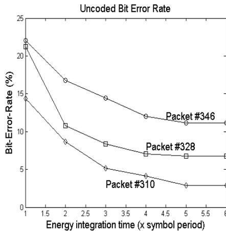
**FIGURE 7.** Uncoded BER vs. Integration Time
