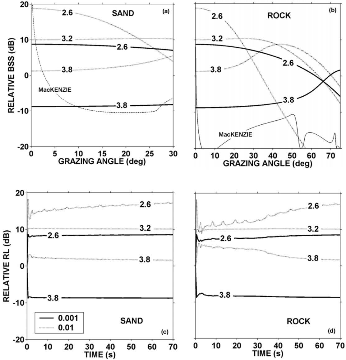
**FIGURE 5.** At 3.5 kHz for sand (left) and rock (right): scattering strengths (top) and reverberation levels (bottom) *relative* to the  $\gamma_2 = 3.2$  and  $w_2 = 0.001 \text{ m}^4$  case. Summer profile, S-R at 75 m. The solid and dotted curves correspond to  $w_2$ 's of 0.001 and 0.01  $\text{m}^4$ , respectively, with the  $\gamma_2$ 's as shown.
