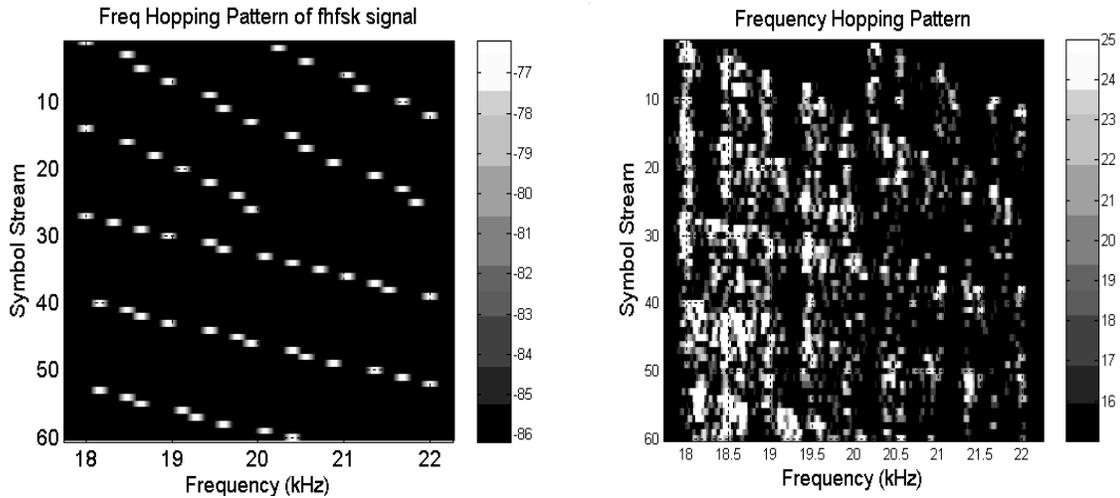
**FIGURE 6.** RDS4 Hopping Pattern (a) Transmit Signal (left figure) and (b) Received Signal (right figure)
