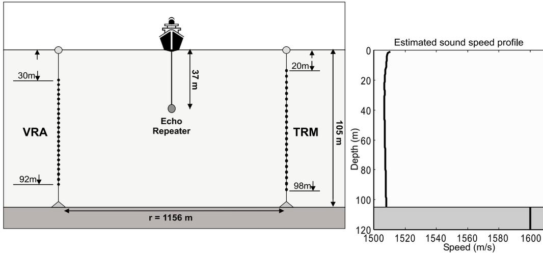
**FIGURE 1.** The experiment configuration, not drawn to scale. The SRA's 29 tx/rx transducers spanned 78 m of the water column. The VRA's 32 hydrophones covered 62 m of the water column. One VRA hydrophone did not function. The two arrays were linked to a common data acquisition point aboard the ship via RF telemetry.
