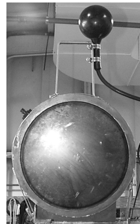
FIGURE 5. Photo of parametric sonar (bottom) and ITC 1001 transducer (top).
