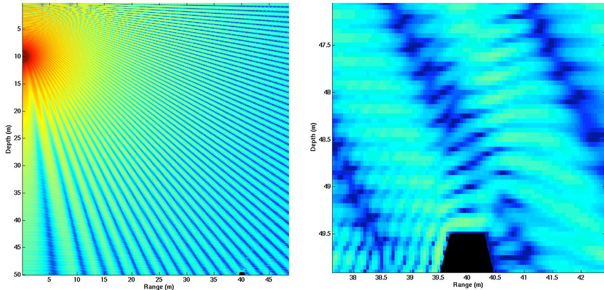
*Figure 2: The pressure field scattered by a truncated cone in a waveguide. The right figure is a close-up of the field in the vicinity of the target.*
