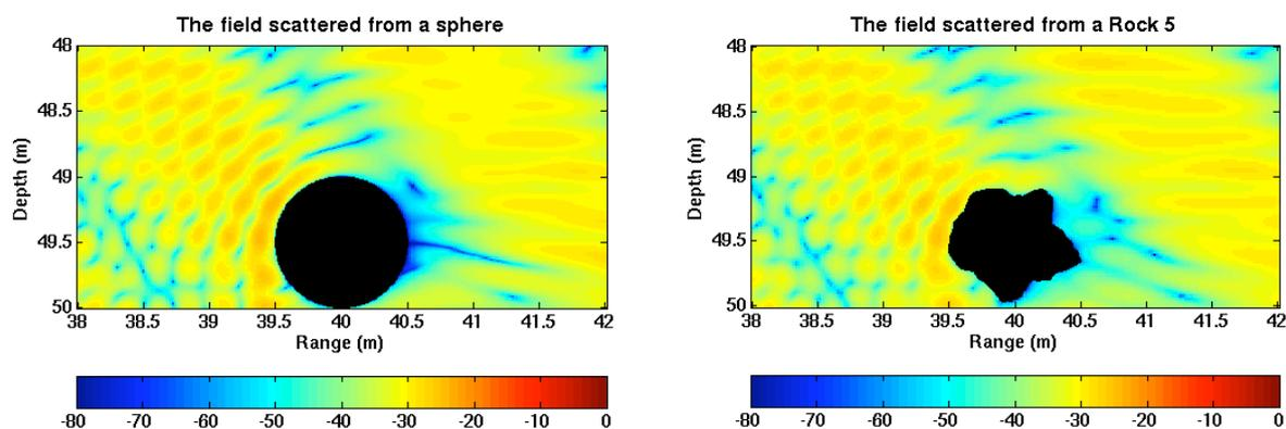
Figure 3: The left panel shows the scattered field in the vicinity of a sphere in a Pekeris waveguide and the right panel shows the same for the rock.
