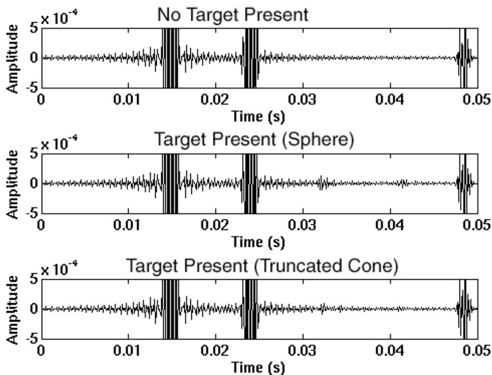
Figure 4: Target echoes in a Pekeris waveguide. The top panel shows the received signal at ( $r=20$  m,  $z=2$  m) in the absence of any target. The middle panel shows the received signal when the sphere is present and the bottom panel shows the same for the rock. Target returns are observed at approximately 32 ms and 42 ms.
