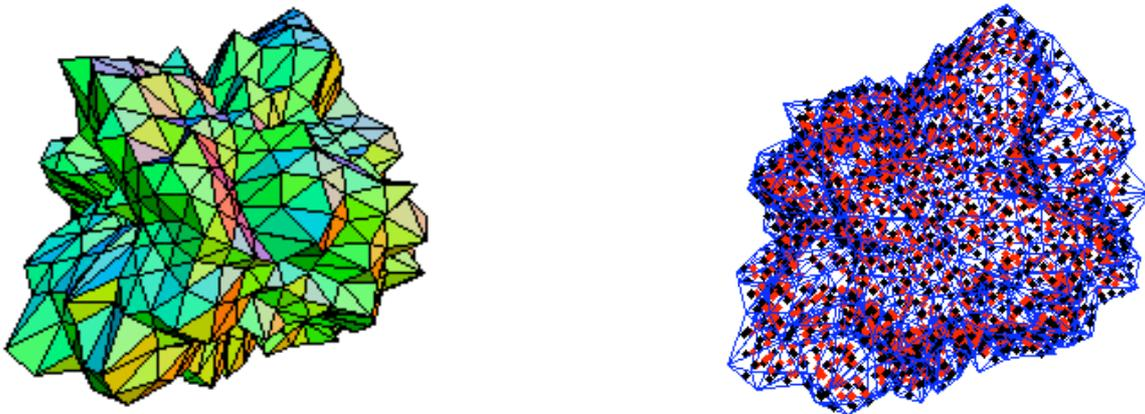
*Figure 1: The figure on the left shows the rock used in one of the examples and the figure on the right shows the distribution of sources (red dots) and nodes (black dots) on its surface.*
